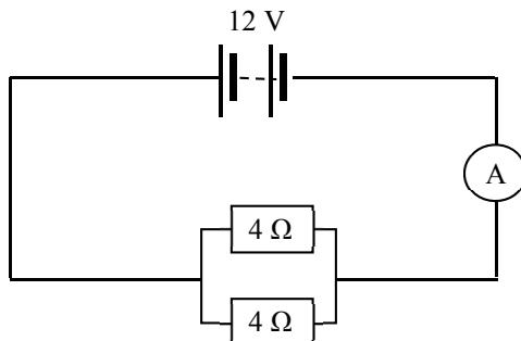
The diagram above shows a circuit with a 12 V d.c. power supply, an ammeter, and two  $4\ \Omega$  resistors connected in parallel.
