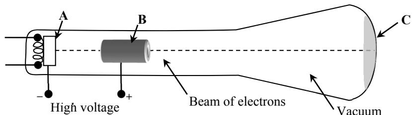
The diagram shows a simple cathode ray tube, which produces a beam of electrons by thermionic emission.
